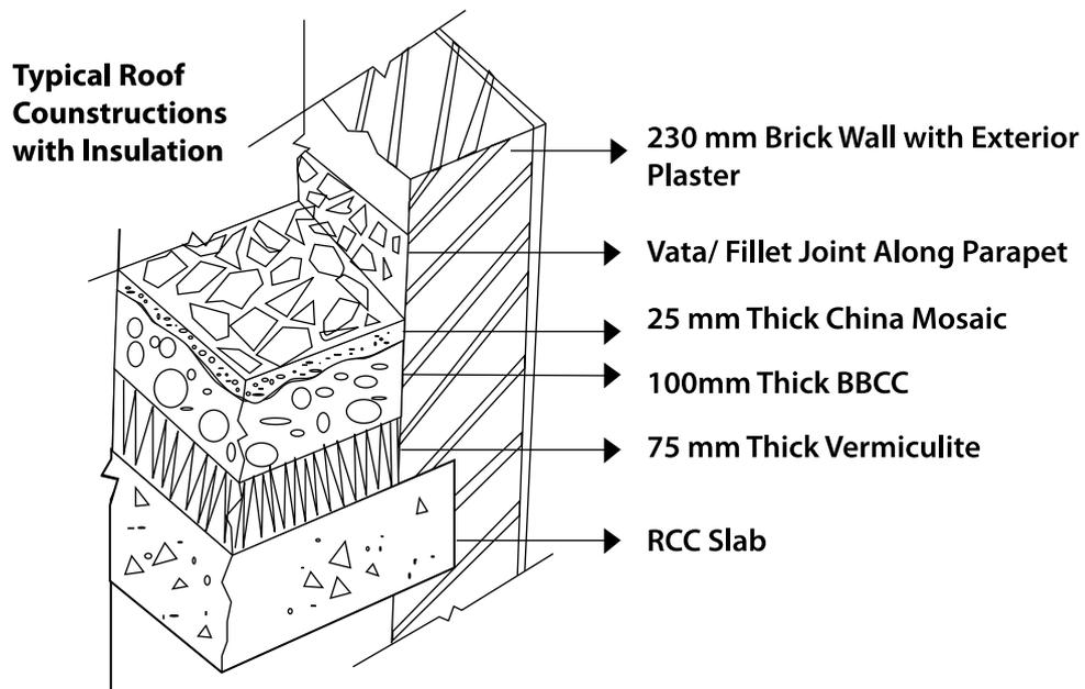
A. RCC Slab Insulated with Vermiculite
