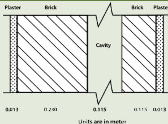
**Figure 4.4: Typical Cavity Wall Construction**
