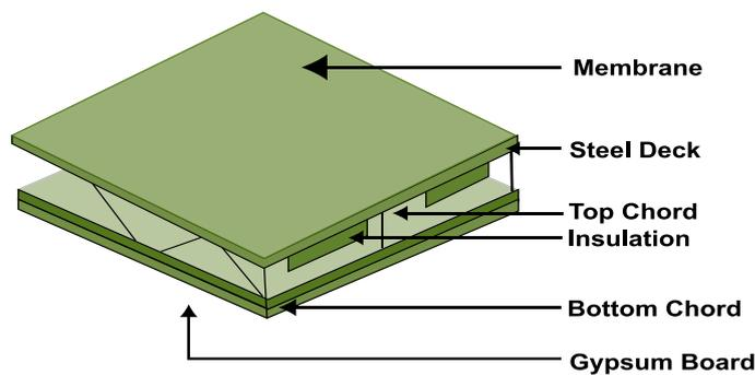
*Steel Joist Roof with Insulated Cavities*
