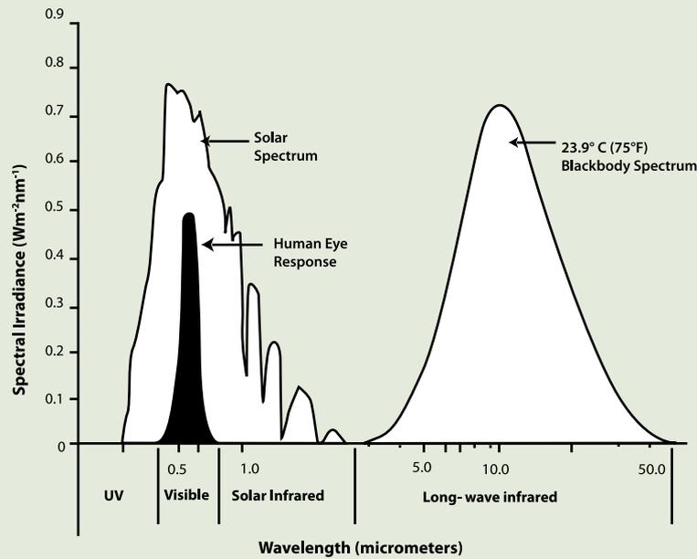
**Figure 4.2: The Solar and Blackbody Spectrum**
