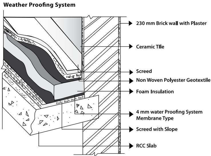
**Figure 4.8: Typical Insulation Technique for RCC Roof Construction**
