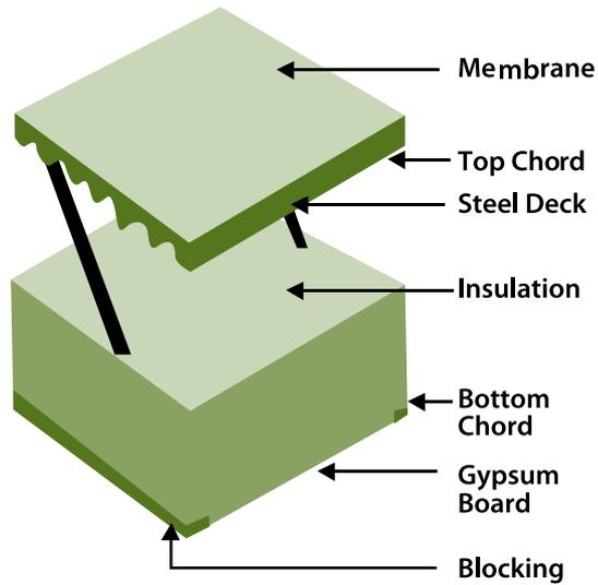
Steel Joist Roof with Continuous Insulation
