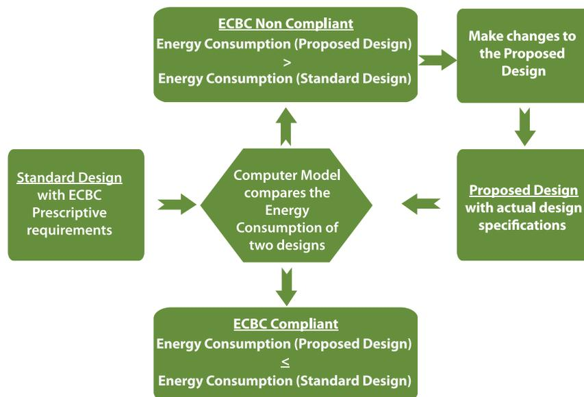
**Figure 3.1: Design Process for the Whole Building Performance Method**
