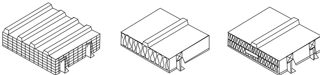
*Pre-Fabricated Metal Roofs Showing Thermal Blocking of Purlins*
