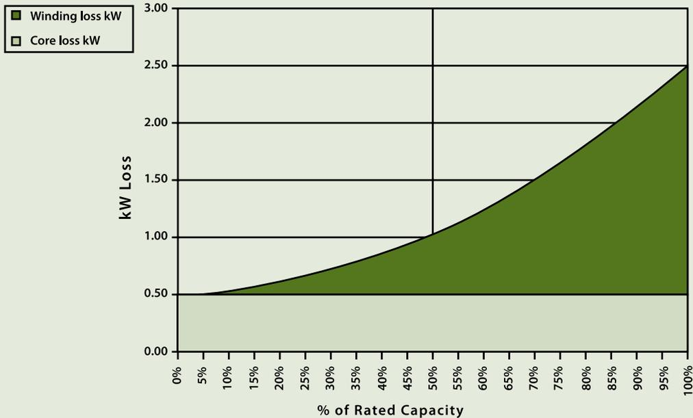
**Figure 8.2: Transformer loss vs % Load**
