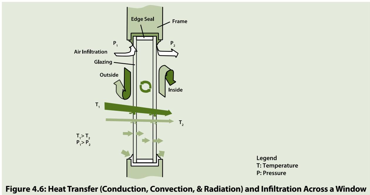
**Figure 4.6: Heat Transfer (Conduction, Convection, & Radiation) and Infiltration Across a Window**
