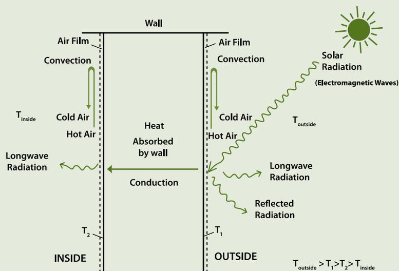
**Figure 4.3: Schematic Showing Three Modes of Heat Transfer**
