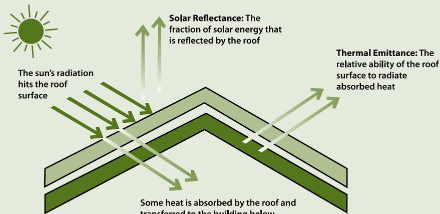
**Figure 4.9: Heat Transfer Through Roof**
