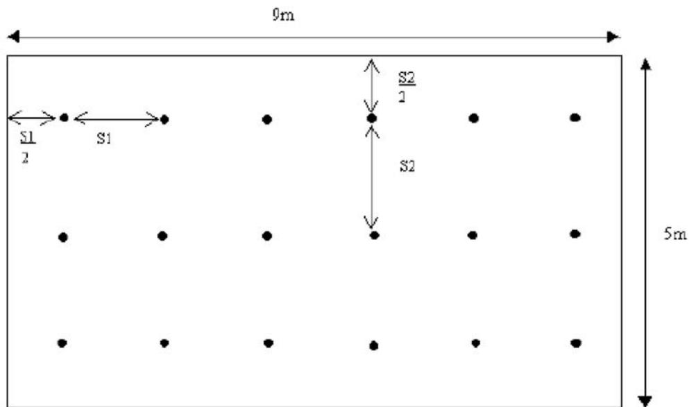
Therefore in this example the spacing between points along rows along the length of the interior =  $9 \div 6 = 1.5\text{m}$  and the distance of the 'end' points from the wall =  $1.5 \div 2 = 0.75\text{m}$ .
